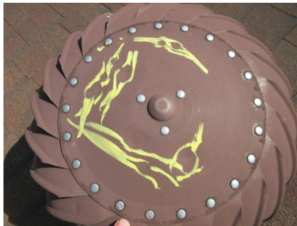
Hail damage to Sam’s roof turbine
